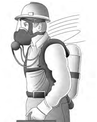
Full Facepiece Self-Contained Breathing Apparatus (SCBA) Pressure demand mode is APF=10,000 Needs to be fit tested
